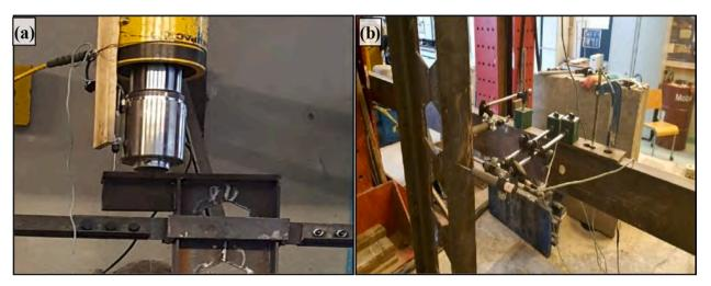
Fig. 7. Arrangment of LVDTs of Groups II&III: (a) Horizontal LVDTs of Groups II&III; (b) Vertical LVDT of Groups II&III.
